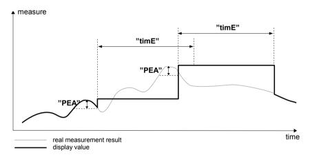
Figure 6.3. Process of peaks detection
