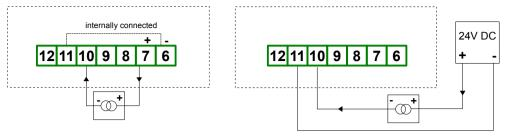
Figure 4.5. Connection of 2-wire current converters
