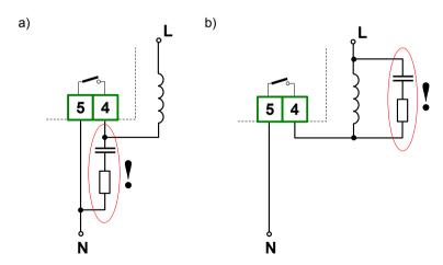
Figure 4.9. Examples of suppression circuit connection:
