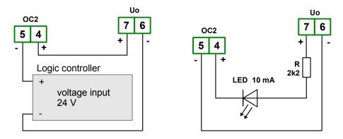
Figure 4.10. Example of OC-type outputs connection
