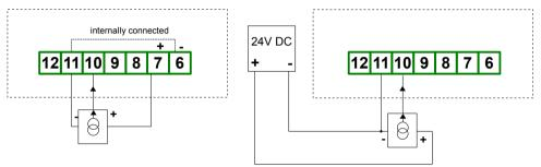
Figure 4.6. Connection of 3-wire current converters
