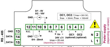
Figure 4.4. Terminals description (OC-type outputs)
