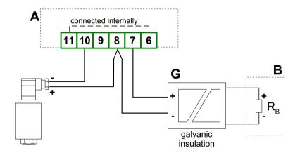
Figure 4.13. Serial connection of passive 2-wire sensor with **PMS-620N** unit and other current measurement device (e.g. PLC controller).
