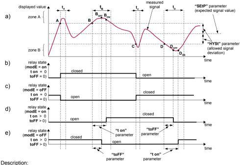
A. B. C. D - points where measured signal exceeds border values (expected value ± allowed deviation)
