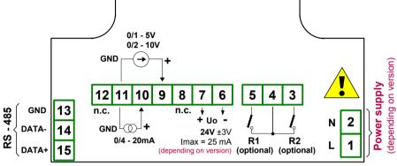
Figure 4.3. Terminals description (relay outputs)
