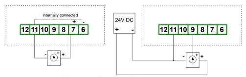
Figure 4.7. Connection of voltage converters
