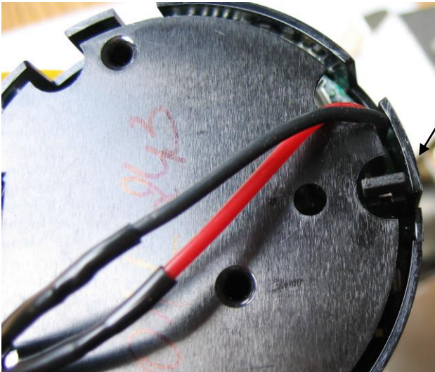
Fig. 6. Jumper of the display backlight unit in the transmitter electronics module (back side of the display).
