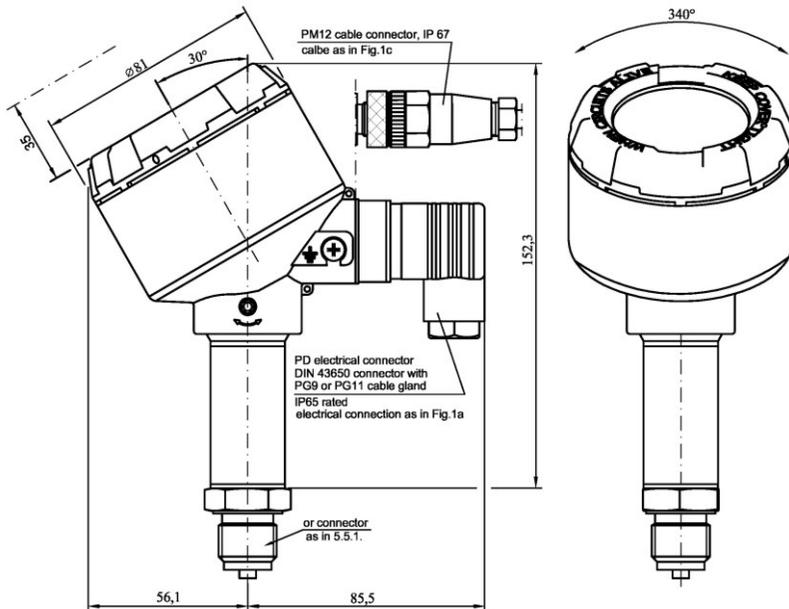
**Figure 3.** PCE-28 transmitter with ALW-type connector:
