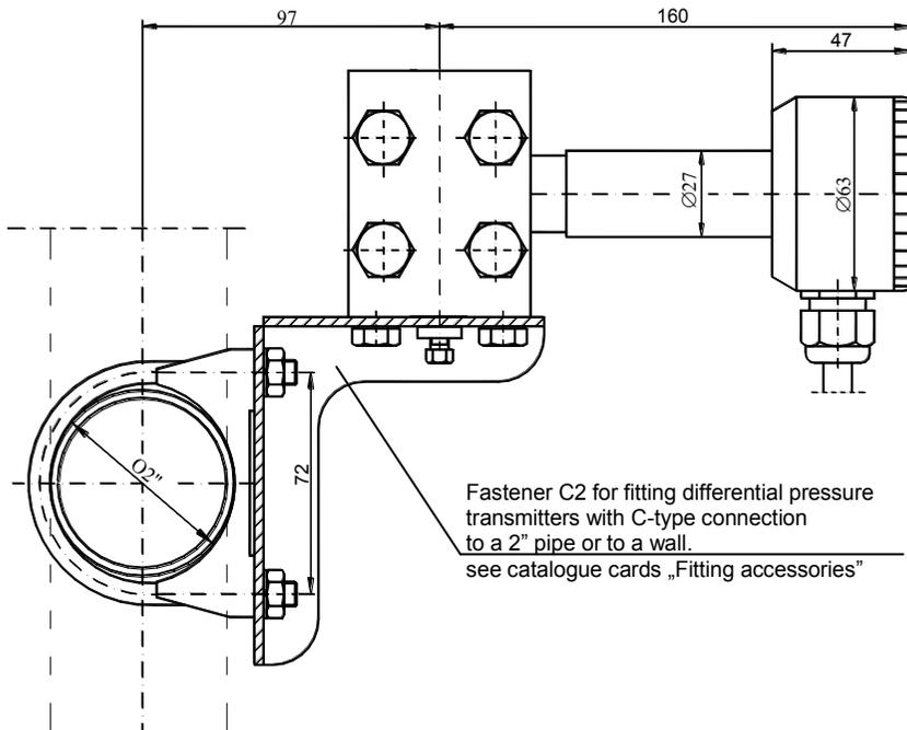
Figure 16. Example: how to install the PRE-28 transmitter on a vertical or horizontal pipe
