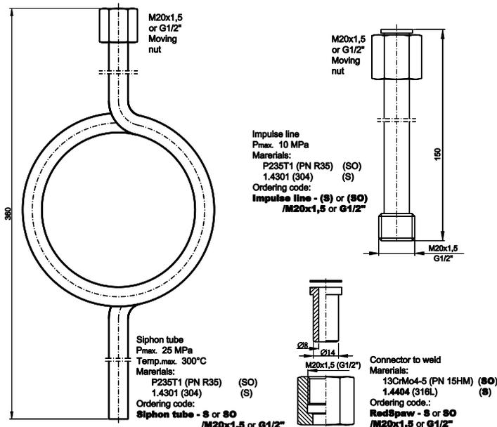
Figure 19. Additional equipment for mounting pressure transmitters.
