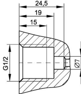
Fig.10b. Socket for use with transmitters with G1/2-type connector
