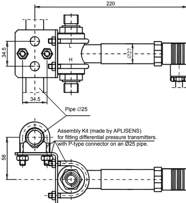
Figure 15. Example: how to install the PRE-28
