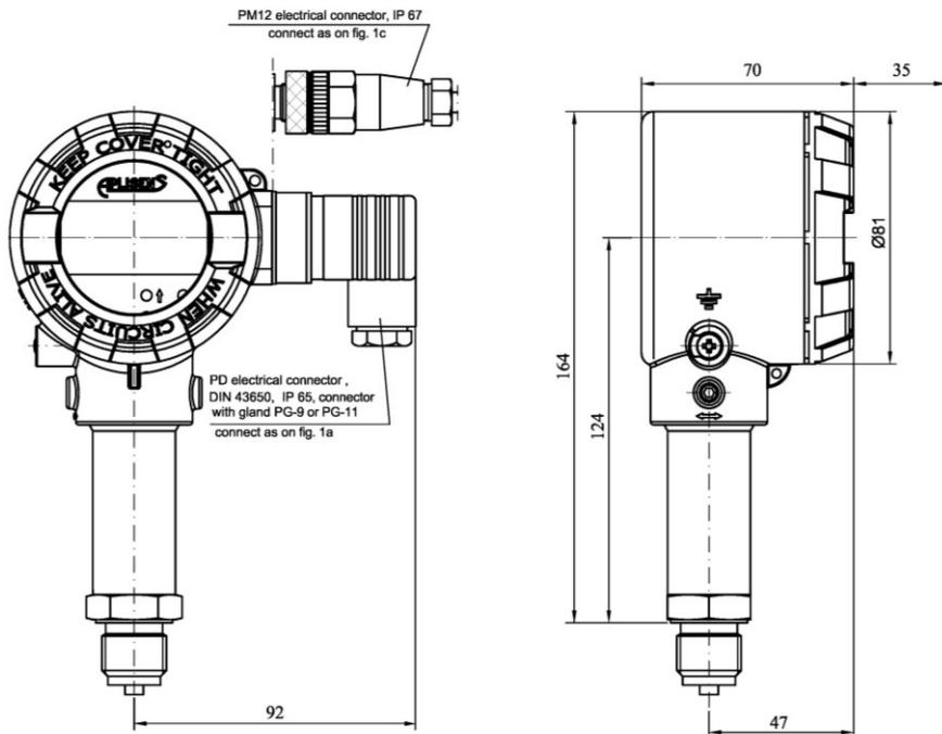
**Figure 4.** PCE-28 transmitter with ALM-type connector:
