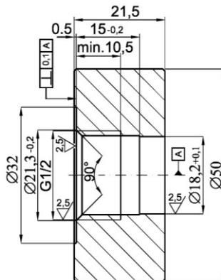
Fig.10d. Weldable fitting ring for use with transmitters with CG1/2 - type connector
