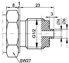
Fig.10a. G1/2-type connector with G1/2" thread
