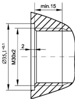
Fig.9b. Socket for CM30x2-type connector
