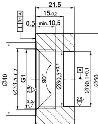
Fig.10f. Weldable fitting ring for use with transmitters with CG1 - type connector
