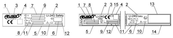
Figure 3. Examples of LI-24G Safety transmitter nameplates in standard and Exi version
