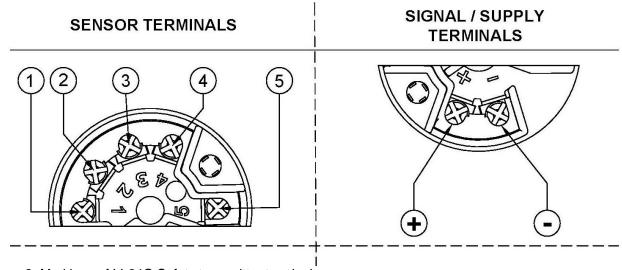
Figure 9. Markings of LI-24G Safety transmitter terminals
