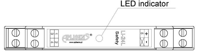
Figure 14. LED indicator on the LI-24L Safety transmitter
