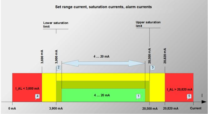
Figure 13. Set range current, saturation currents, alarm currents
