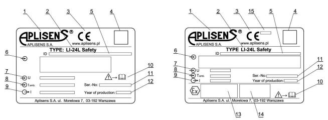
Figure 4. Examples of LI-24L Safety transmitter nameplates in standard and Exi version
