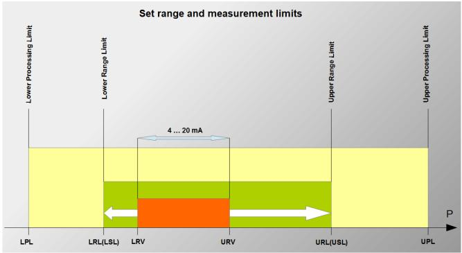
Figure 1. Set range and measurement limits
