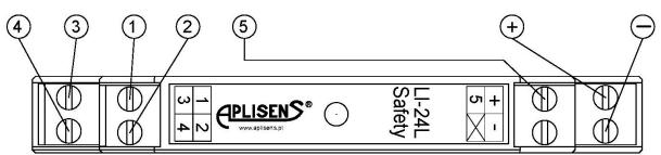
Figure 8. Markings of LI-24L Safety transmitter terminals
