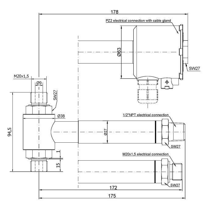
**Figure 2**. Pressure transmitter PRE-28, PRE-28 Ex Safety, PRE-28.Smart, PR-29A, PR-29B, PRE-28.Modbus. Dimensions.
