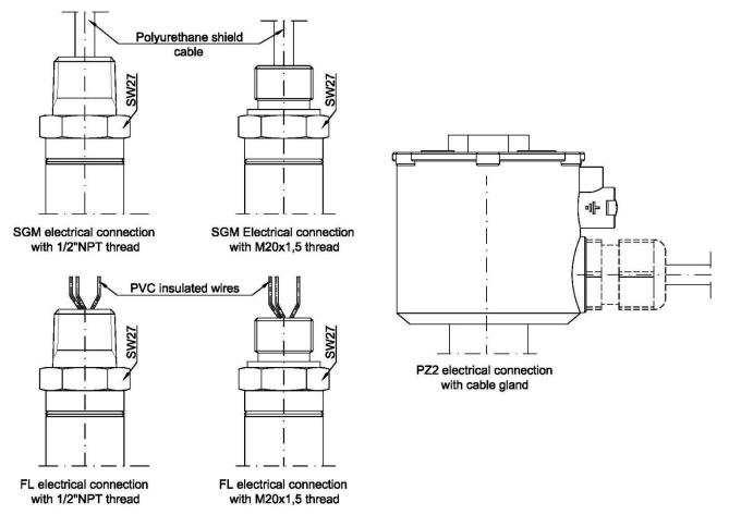
**Figure 3**. Electrical connections of the transmitters PC(R)E-28, PC(R)E-28 Ex Safety, PC(R)E-28.Smart, PC(R)-29A, PC(R)-29B, PC(R)E-28.Modbus.
