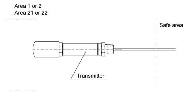
Figure 5. Transmitter installed in the hazard zones
