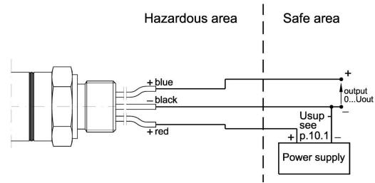
Figure 11. Wiring diagram transmitters PC-29A, PR-29A, PC-29B, PR-29B.
