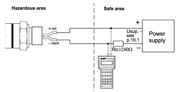
Figure 10. Wiring diagram transmitters PCE-28.Smart, PRE-28.Smart.
