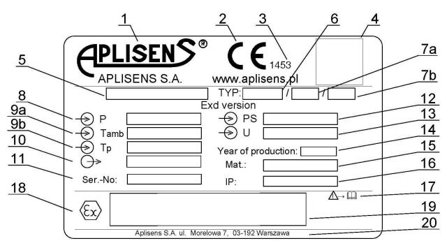
**Figure 4**. PC(R)E-28, PC(R)E-28.Smart, PC(R)-29A, PC(R)-29B, PC(R)E-28.Modbus rating plate (example).
