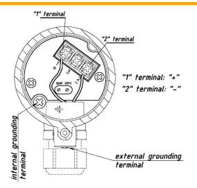
**Figure 6**. Connection of the PCE-28, PRE-28, PCE-28.Smart, PRE-28.Smart, PCE-28 Ex Safety, PRE-28 Ex Safety transmitters with a PZ2 connector.
