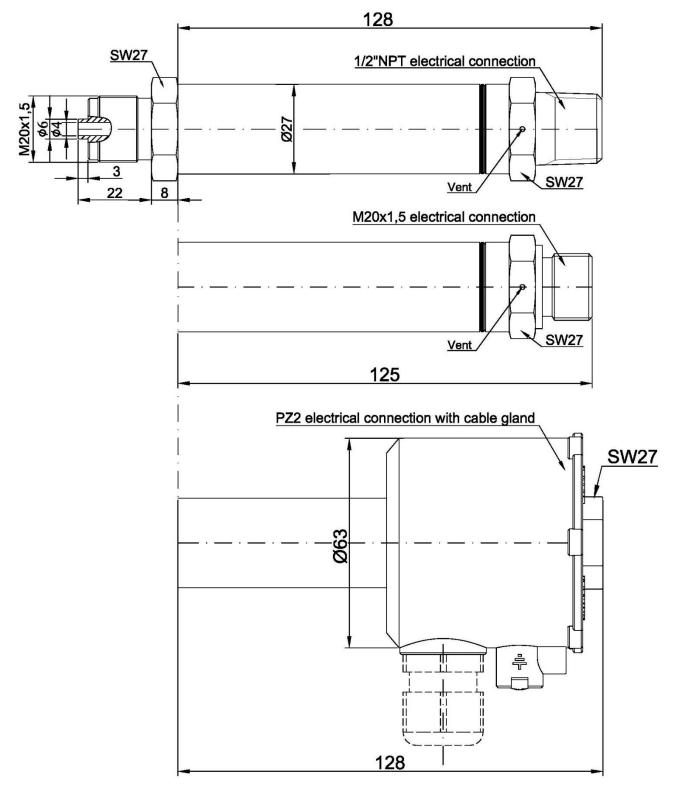
**Figure 1**. Pressure transmitter PCE-28, PCE-28 Ex Safety, PCE-28.Smart, PC-29A, PC-29B, PCE-28.Modbus. Dimensions.
