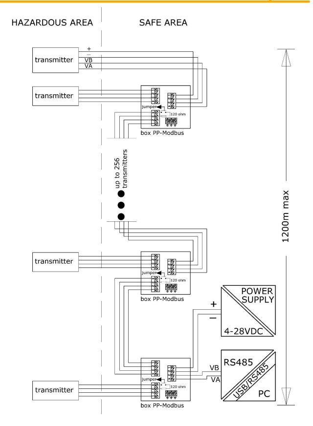
Figure 12. PCE-28.Modbus, PRE-28.Modbus electrical connection.
