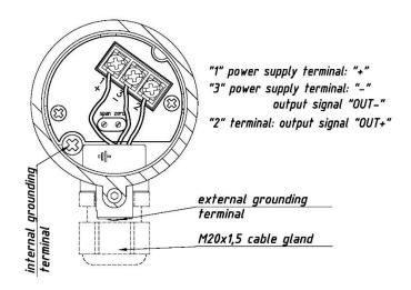
Figure 8. Electrical connection of the PC-29A, PR-29A, PC-29B, PR-29B transmitters with a PZ2 connector.
