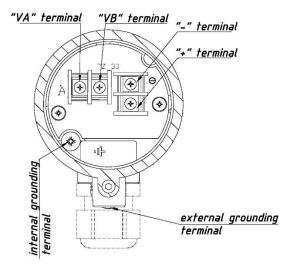
Figure 7. Electrical connection of the PCE-28.Modbus, PRE-28.Modbus transmitters with PZ2 type connection.
