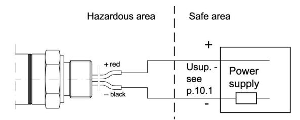
Figure 9. Wiring diagram transmitters PCE-28, PRE-28, PCE-28 Ex Safety, PRE-28 Ex Safety.
