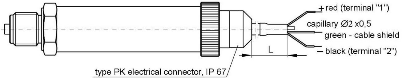
**Figure 3.** Connection of the transmitter with PK electrical connector
