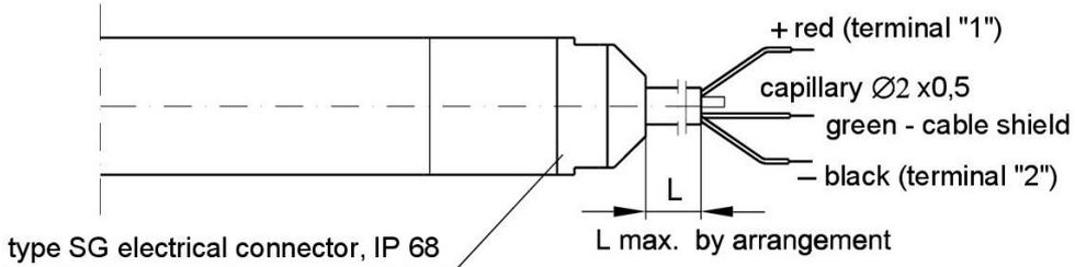
**Figure 5.** Connection of the transmitter with SG electrical connector
