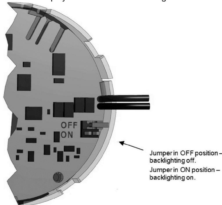
**Figure 4.** Backlighting jumper view at transmitter electric board (unit display back side)
