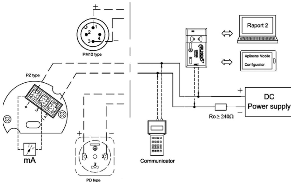
**Figure 2.** Electrical connection 4...20 mA of HART to transmitter in standard version
