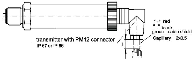
**Figure 5.** Connection of the transmitter with PM12 electrical connector
