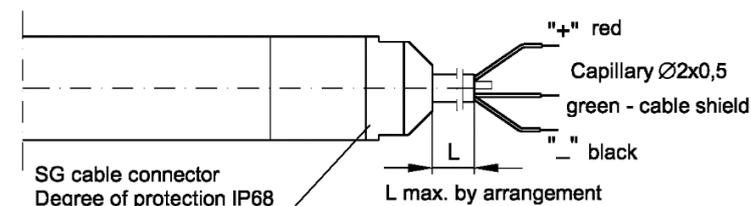
**Figure 4.** Connection of the transmitter with SG electrical connector
