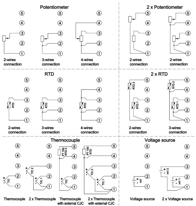
Figure 9. Possible ways of sensor connection
