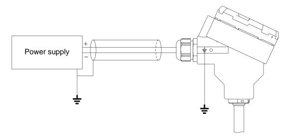
Figure 12. The recommended way to connect earthing for LI-24G transmitter in the connection head
