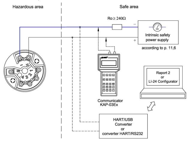
Figure 11. Electrical connection the LI-24G transmitter in the hazardous area
