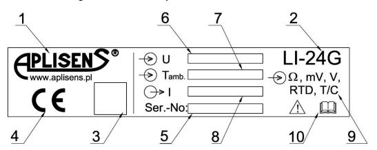
Example of the rating plate of LI-24G transmitter in normal version
