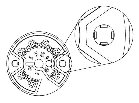
Figure 7. Protect against the fastening screws falling out
