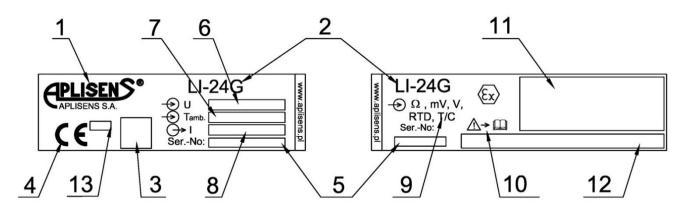
Example of the rating plate of LI-24G transmitter in Ex version
