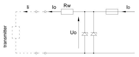
Figure 14. Linear power supply configuration
