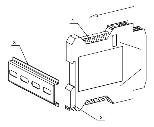
Figure 5. Mounting the LI-24L transmitter on DIN 35 rail
