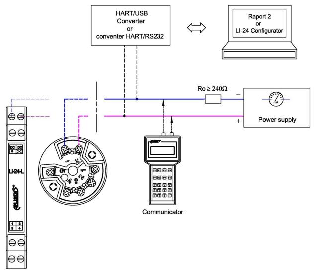
Figure 10. Electrical connection the transmitter in the safe areas
