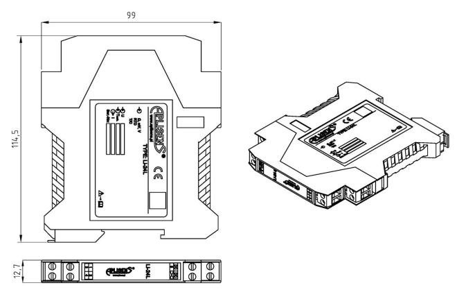
Figure 2. The LI-24L temperature transmitter. Dimensions
